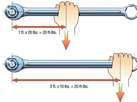
Torque is measured in units of distance multiplied by force. A force of 10 lb. – acting through a distance of 2 feet – produces exactly the same torque, 20 ft.-lb., as a force of 20 lb. – acting through a distance of 1 foot.
